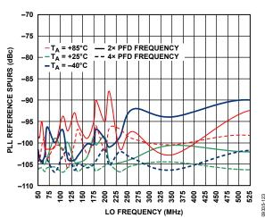
Figure 23. PLL Reference Spurs vs. LO Frequency
