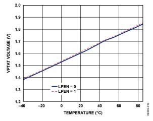
Figure 19. VPTAT vs. Temperature
