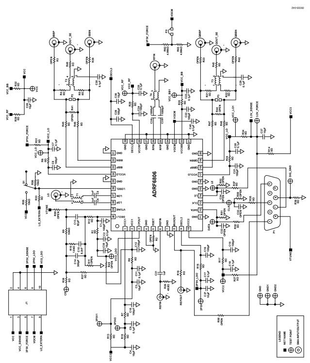
Figure 44. Evaluation Board Schematic
