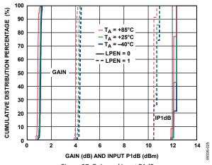
Figure 27. Gain and Input P1dB
