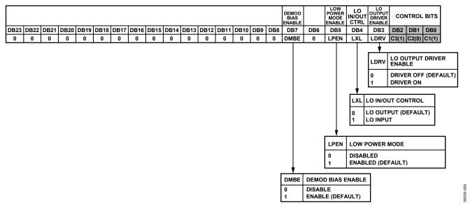
Figure 38. LO Path and Demodulator Control Register (R5)
