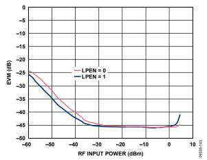
Figure 43. EVM Measurements @ 140 MHz 256 QAM; Symbol Rate = 5 MHz; BB IF Frequency of 5 MHz
