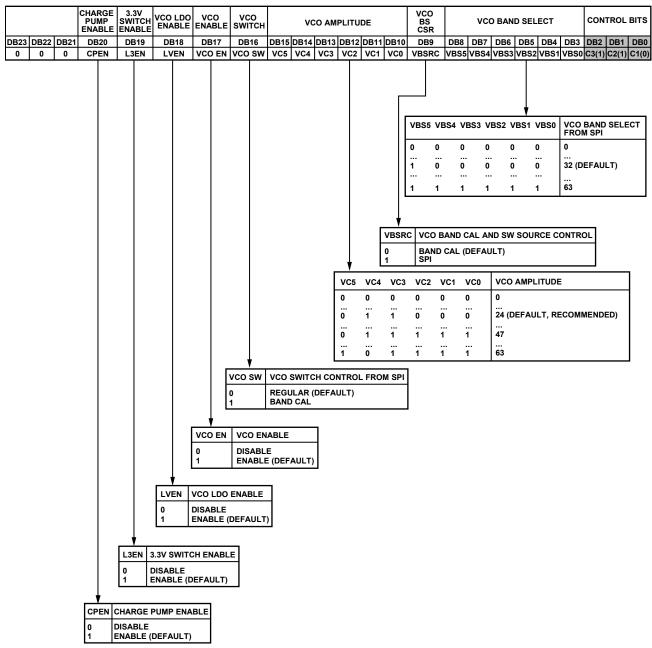
Figure 39. VCO Control and Enables (R6)
