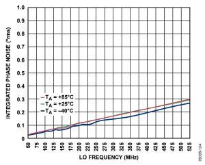
Figure 24. Integrated Phase Noise vs. LO Frequency (Spurs Omitted)
