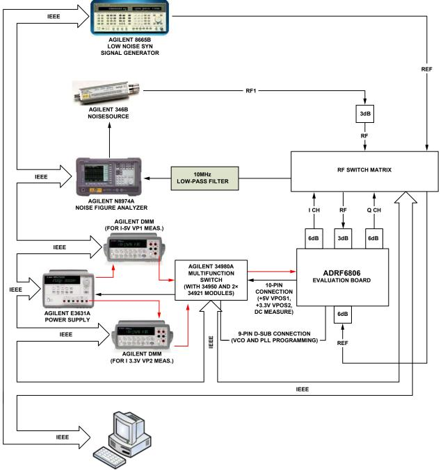
Figure 51. Noise Figure Characterization Setup
