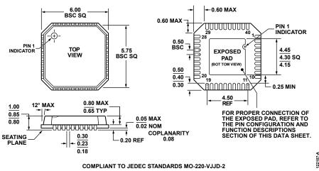
Figure 53. 40-Lead Lead Frame Chip Scale Package [LFCSP\_VQ] 6 mm × 6 mm Body, Very Thin Quad (CP-40-4) Dimensions shown in millimeters
