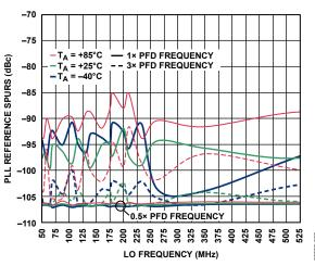
Figure 22. PLL Reference Spurs vs. LO Frequency
