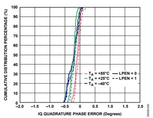
Figure 32. IQ Quadrature Phase Error
