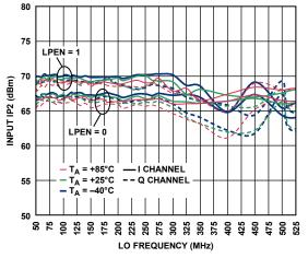
Figure 7. Input IP2 vs. LO Frequency
