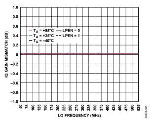
Figure 6. IQ Gain Mismatch vs. LO Frequency
