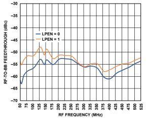
Figure 12. RF-to-BB Feedthrough vs. RF Frequency
