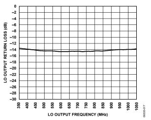
Figure 17. LO Output Return Loss vs. LO Output Frequency, LO Output Enabled (350 MHz to 1050 MHz)
