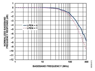
Figure 13. Normalized BB Frequency Response
