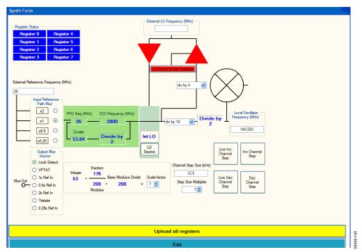
Figure 49. Evaluation Board Software Synth Form Window
