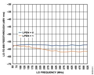
Figure 11. LO-to-BB Feedthrough vs. LO Frequency, LO Output Turned Off
