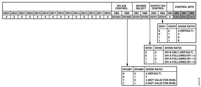
Figure 40. LO Divider Control Register (R7)
