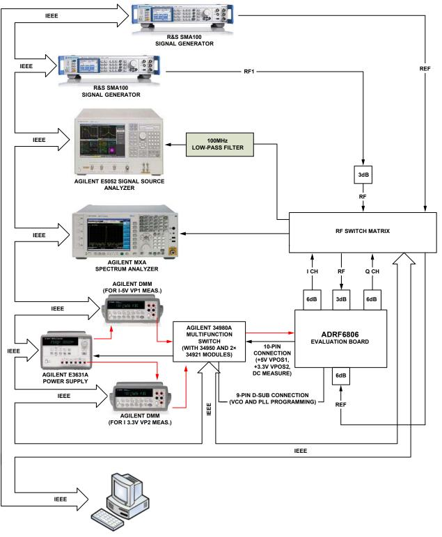
Figure 52. Phase Noise Characterization Setup
