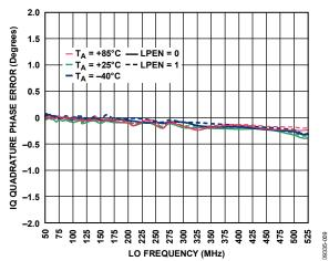
Figure 9. IQ Quadrature Phase Error vs. LO Frequency
