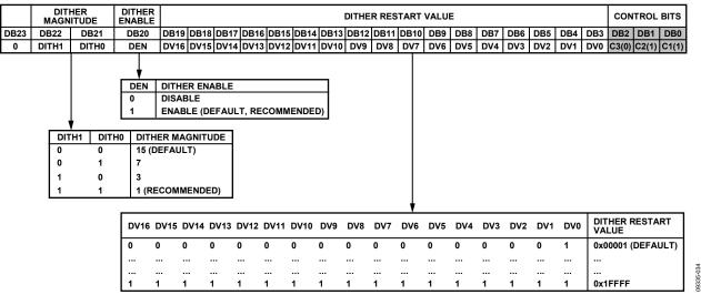
Figure 36. Σ-Δ Modulator Dither Control Register (R3)
