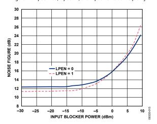
Figure 15. Noise Figure vs. Input Blocker Level,  $f_{LO} = 140 \text{ MHz}$  (RF Blocker 5 MHz Offset)
