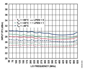
Figure 5. Input IP3 vs. LO Frequency
