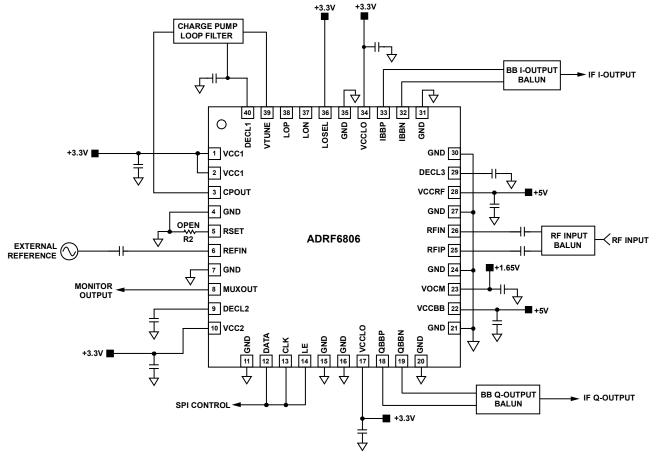
Figure 41. Basic Connections
